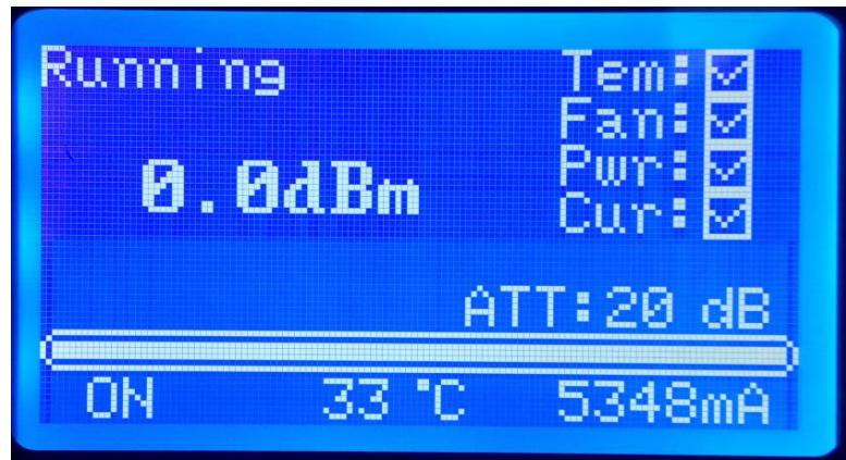
In the event of over-temperature, over-current and/or fan failure, the amplifier will be locked in the protection mode and alarm information will be displayed on the LCD (see below image).
